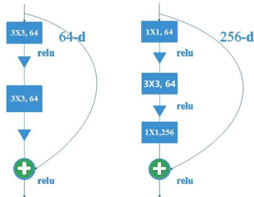
Figure 1. Schematic diagram of the residual block model
