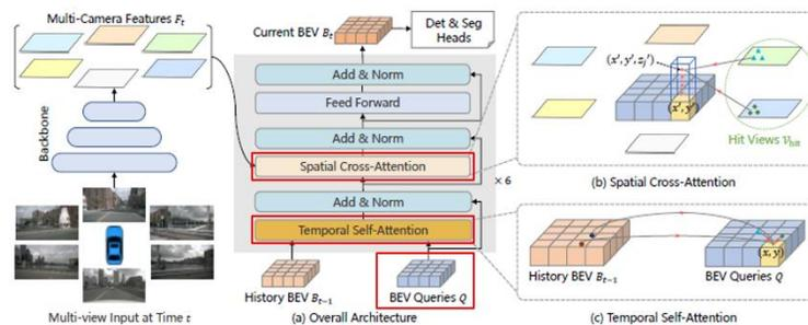
**Figure 4. BEVFORMER model Principle structure diagram(Li, Z ed at., 2022 )**
